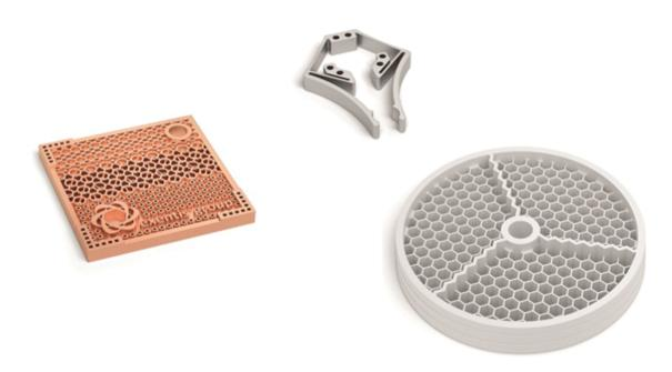
A copper sample part (left), a metallic forcep for medical applications (centre) and a casting filter for lowpressure casting of aluminium rims (right) (Courtesy Exentis Group AG)
