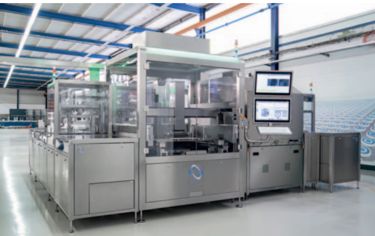
Exentis Pharma production system for the manufacturing of tablets with a freely adjustable release profile of active ingredients in the human body
